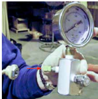
Attaching hose/gas chuck to gas valve; remove yellow safety cap; thread gas chuck to .305-32 Valve stem — DO NOT OVERTIGHTEN
